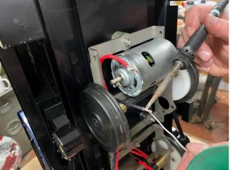
The motors have two teminals, one has a red dot on it to signify positive. The colour wire you chose to position on this red dot is not important, what is important is repeating this choice on each motor to ensure they are uniform. Failiure to do this will result in motors running in alternate directions.
