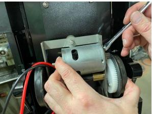
Trim the cables back so they have an easy run to the motors. Strip the insulation back about 6mm on each cable and push the end through the brass tab on the back of the motor, soldering on the cable.
