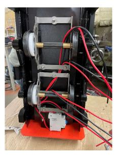
Each motor requires one red and one black wire, take care to position the wires away from any moving parts. including the wheel sets, also avoiding making sharp kinks in the wires as these can overheat when drawing amps at low revs.
