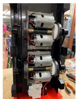
Lubricate the chassis, Vaseline the gears. This is a good time to check the body work and bolts as the models do get shaken about in transit and you may find some bolts work their way loose, tighten any you find. You can apply Loctite to prevent them loosening again if you wish. If you are missing bolts, please contact Maxitrak for spares.
